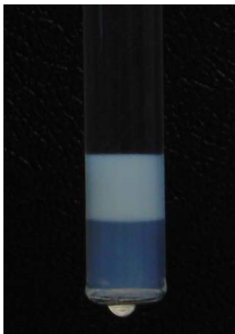
Figure 3.9: A photo showing the three coexisting macroscopic phases for the sample of 0.2 wt% HMHEC+4 wt% TX100.
