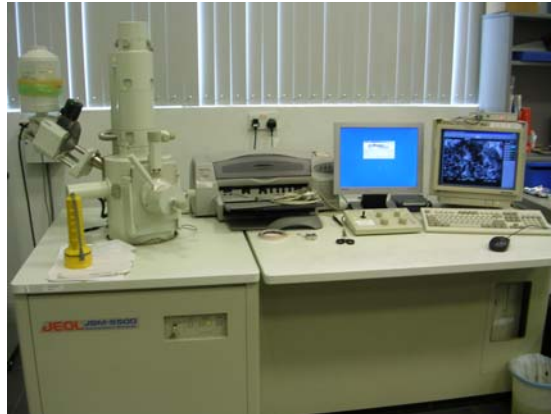
Figure 3.5 JEOL JSM-5500 Scanning Electron Microscope.
