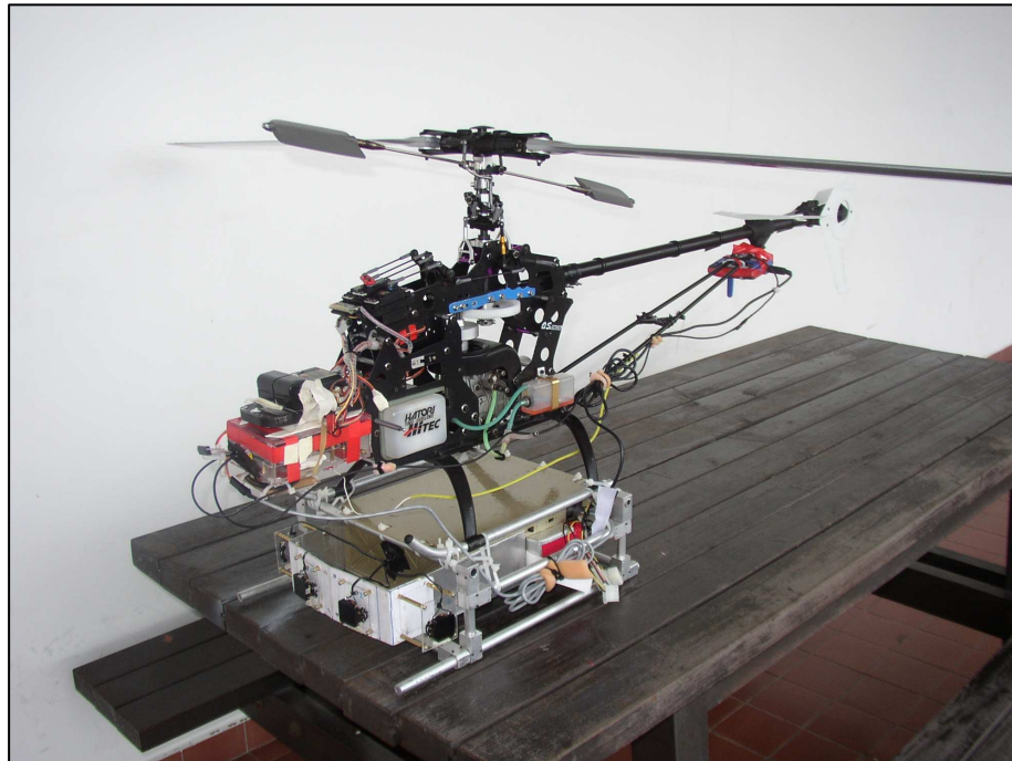
Figure 4.1: UAV Flight Computer Mounted
