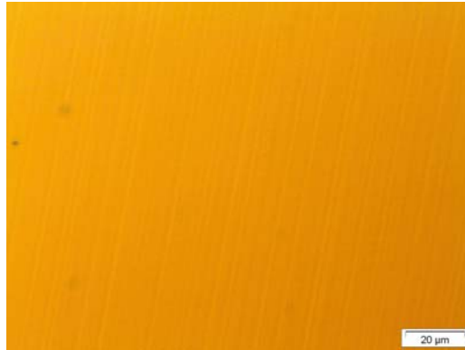
Figure 4.7.a Fracture free surface at a_0 100nm f 2 \mu m/rev D_{max} 19 nm.
