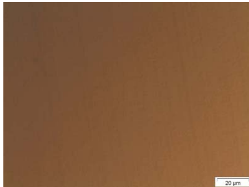
Figure 4.9.a Fracture free surface at a_0 150nm f 1.5 \mu\text{m}/\text{rev} D_{\text{max}} 24.85 nm.
