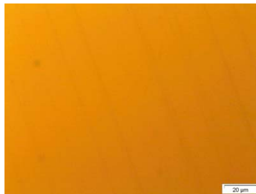
Figure 4.6.b Fracture free surface at a_0 80nm f 2 \mu\text{m}/\text{rev} R 2mm D_{\max} 17 nm.
