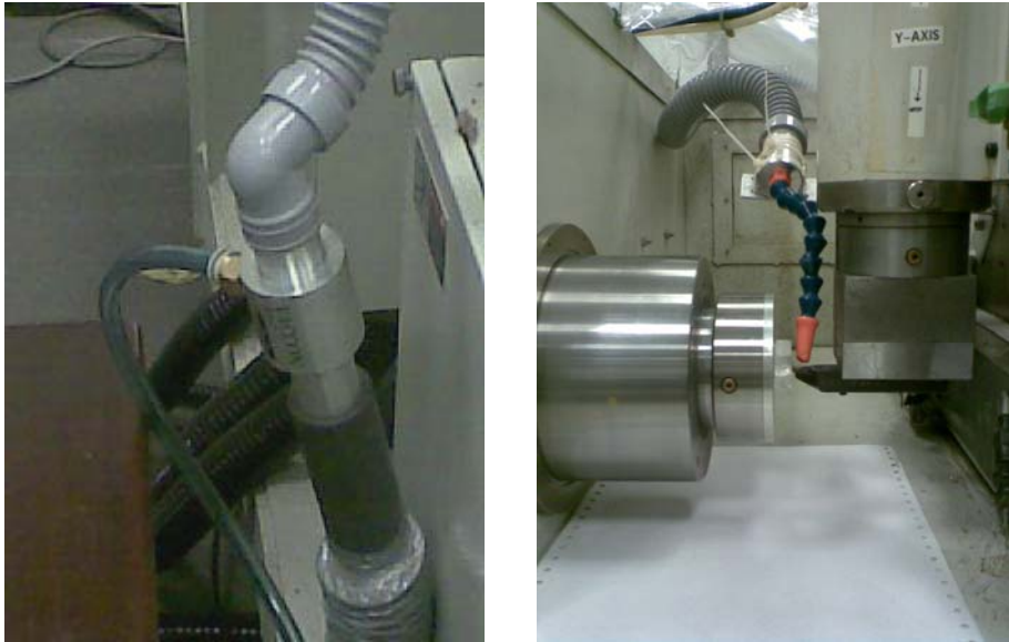
Figure 3.7 Venturi vacuum setup and nozzle near work zone.
