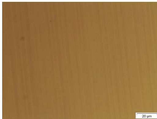
Figure 4.8.a Fracture free surface at a_0 100nm f 1.5 \mu m/rev D_{max} 20 nm.
