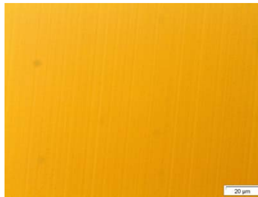
Figure 4.6.a Fracture free surface at a_0 80nm f 2 \mu\text{m}/\text{rev} R 2mm D_{\max} 17 nm.
