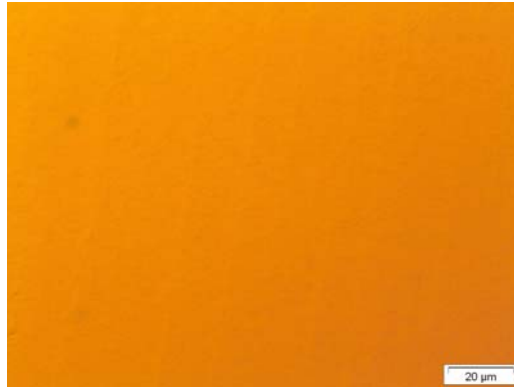
Figure 4.7.b Fracture free surface at a_0 100nm f 2 \mu m/rev D_{max} 19 nm.
