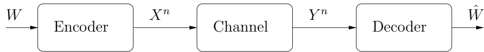
Figure 2.2: Basic single user communication channel. The channel is represented by a conditional probability mass function p(y^n|x^n) . The encoder maps each message into a codeword x^n . Inversely, the decoder maps the channel output y^n into a message estimate.
