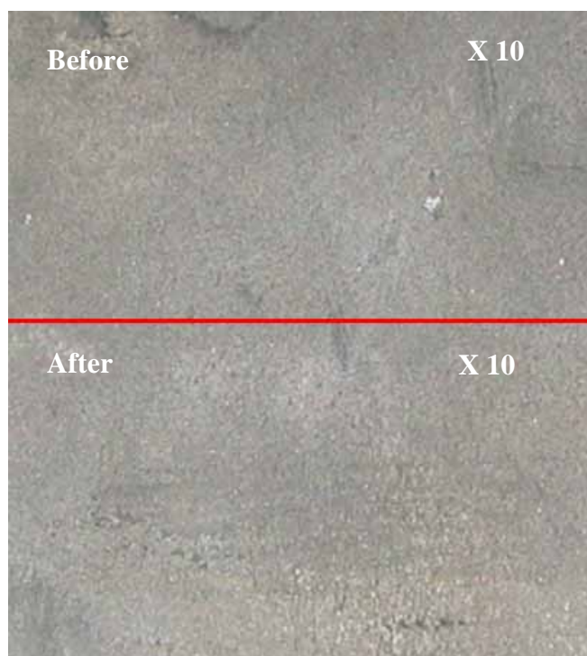
Figure. 6.9 Microscopic views of the Ni plated PDMS surface before and after the peel test
