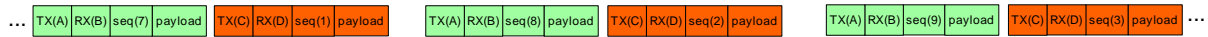
Figure 6.1: Detecting packet collision via an interleaved fragment sequence, where TX/RX IDs are alternate and seq 's are inconsecutive .
