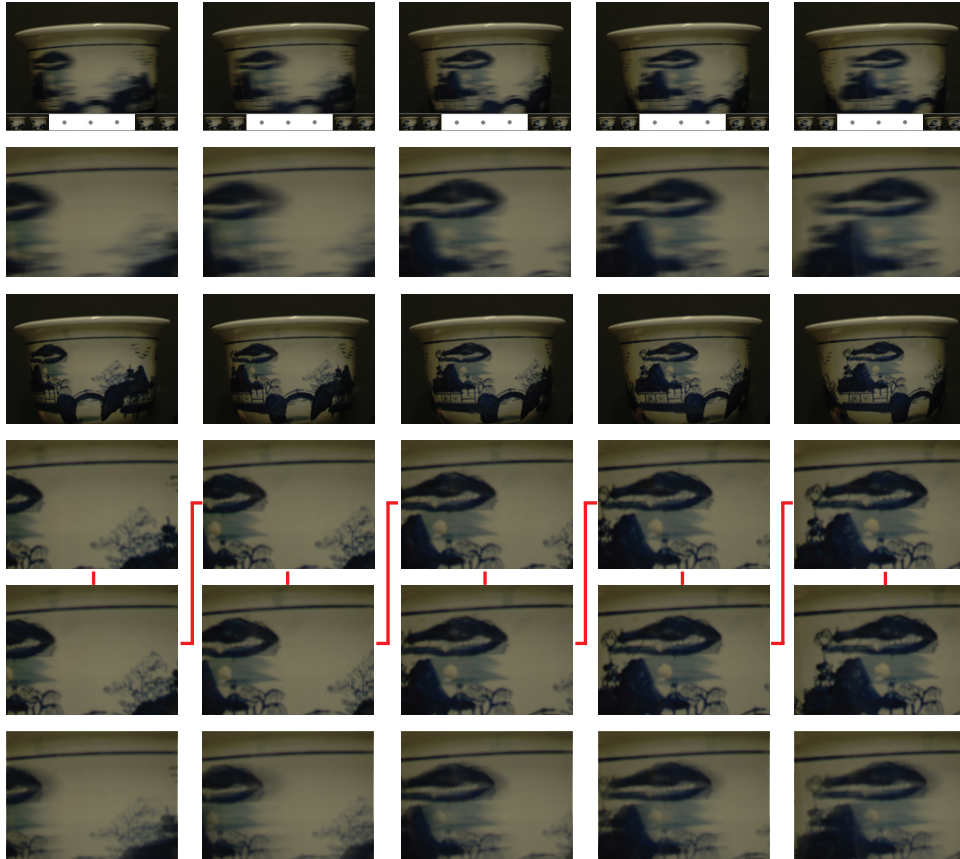
Figure 4.18: Video deblurring with out-of-plane rotational motion. The moving object is a vase with a center of rotation approximately aligned with the image center. First Row: Input video frames. Second Row: Close-ups of a motion blurred region. Third Row: Deblurred video. Fourth Row: Close-ups of deblurred video using the first low-resolution frames as the reference frames. Fifth Row: Close-ups of deblurred video frames using the fifth low-resolution frames as the reference frames. The final video sequence has higher temporal sampling than the original high-resolution video, and is played with frames ordered according to the red lines. Bottom row: Results from space-time super-resolution [34].
