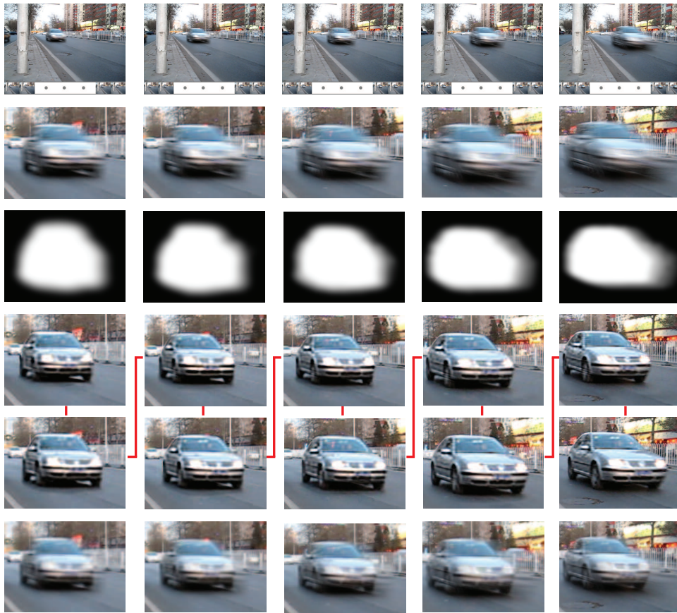
Figure 4.20: Video deblurring in an outdoor scene. The moving object is a car driving towards the camera, which produces both translation and zoom-in blur effects. First Row: Input video frames. Second Row: The extracted alpha mattes of the moving object. Third Row: The deblurred video frames using the first low-resolution frames as the reference frames. Fourth Row: The deblurred video frames using the third low-resolution frames as the reference frames. The final video consists of frames ordered as indicated by the red lines. By combining results from using different low-resolution frames as reference frames, we can increase the frame rate of the deblurred video. Bottom row: Results from space-time super-resolution [34].
