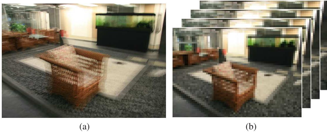
Figure 4.1: Tradeoff between resolution and frame rates. (a) Image from a high-resolution, low-frame-rate camera. (b) Image from a low-resolution, high-frame-rate camera.
