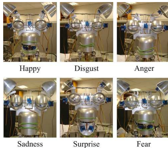
Figure 6.3: The robotic face is able to show its emotions through facial features situated in the frontal part of the head. The figure illustrates the features' configuration for each universal expression.
