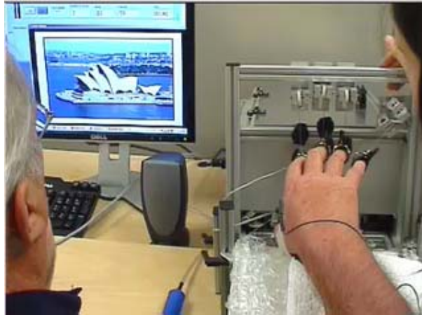
Fig.3.4 Post-stroke subject performing hand close-open motion with robotic device
