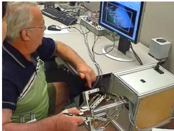
Fig.3.5 Post-stroke subject performing forearm pronation-supination motion with robotic device
