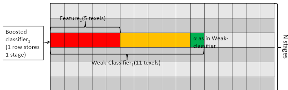
Figure 4.2: GPU-based classifier cascade texture: updated every pass to adapt fractional re-scaling.
