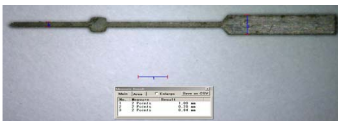
Figure 7.7: High aspect ratio second hand needle of 20 \mu\text{m} Magnification: 50X
