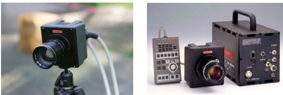
Figure 4.5: High speed camera utilized in the research work for capturing the vibration of the wire electrode
