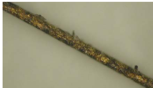
Figure 4.4: Tungsten wire after machining. The wear of the wire is clearly visible in the photograph.
