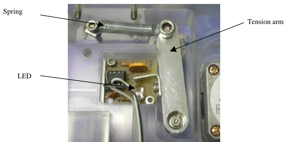
Figure 3.5: Photograph of the tension arm mechanism
