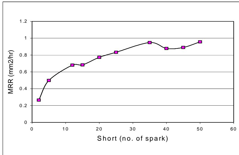
Figure E.2: Effect of short detection parameter on material removal rate
