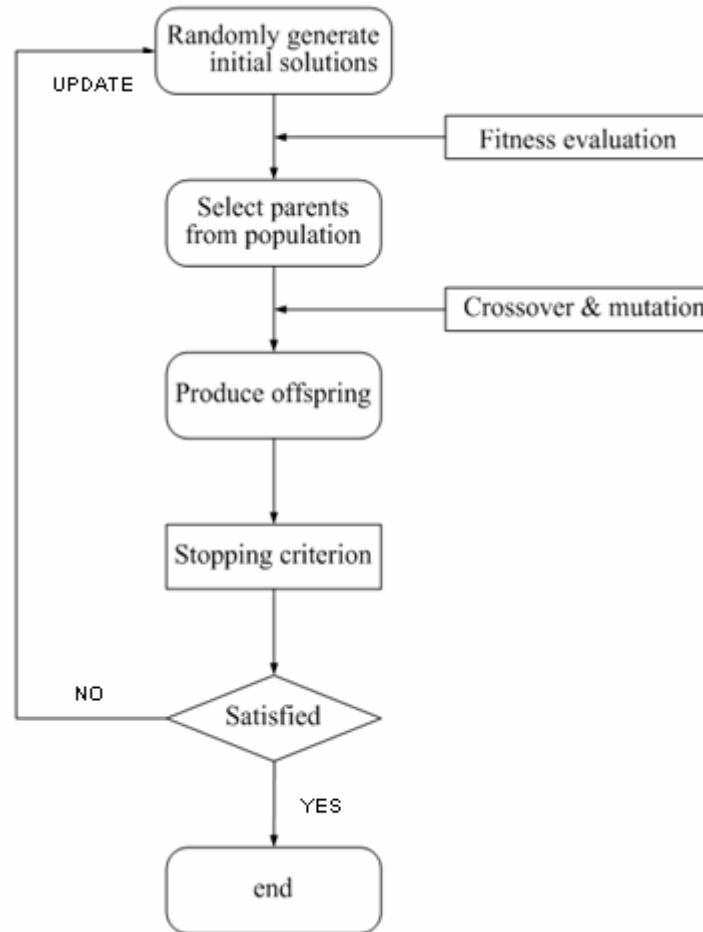
Figure 2.3 An Illustration of the Process of Genetic Algorithm.
