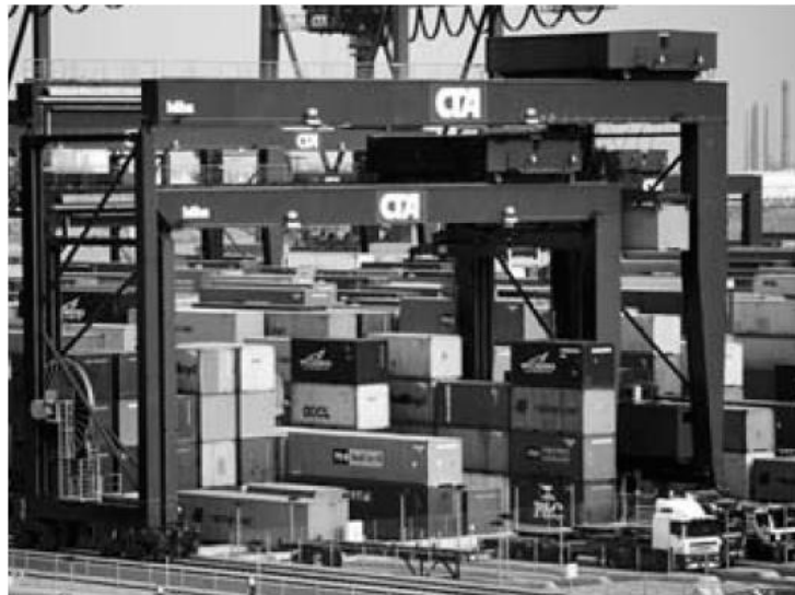
Figure 6.1 A DRMG System in Operation (Steenken et al., 2004)
