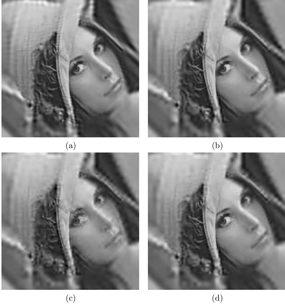
Figure 3.4: Rotated images: (a) J_1 obtained by rotating the foveated image Figure 3.1 (b); (b) J_2 obtained by applying DWT on J_1 and IDWT on the coefficients in the mask; (c) A_1 obtained by Algorithm 1; (d) A_2 obtained by Algorithm 2.
