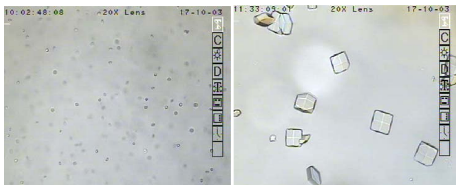
Figure 3.12 (a) The formation of tiny crystals upon cooling at 0.05^{\circ}\text{C}/\text{min} ; (b) the tiny crystals grew to bigger crystals
