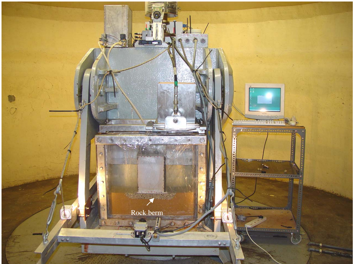
Fig. 3.5 Photograph of centrifuge package setup with rock berm underneath caisson base
