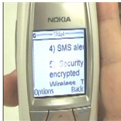
Figure 3.14: Using the zoom function, the processed image is enlarged.
