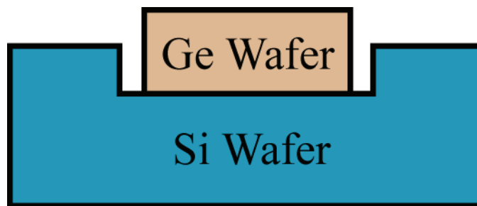
Figure 2.1 Sample configuration for CVD high-k deposition. The Ge wafer is placed on a grooved 6-inch silicon wafer to deposit HfO 2 in a 6-inch single-wafer MOCVD reactor.
