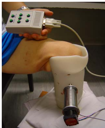
Figure 3.6. Leg position of amputee during indentation test
