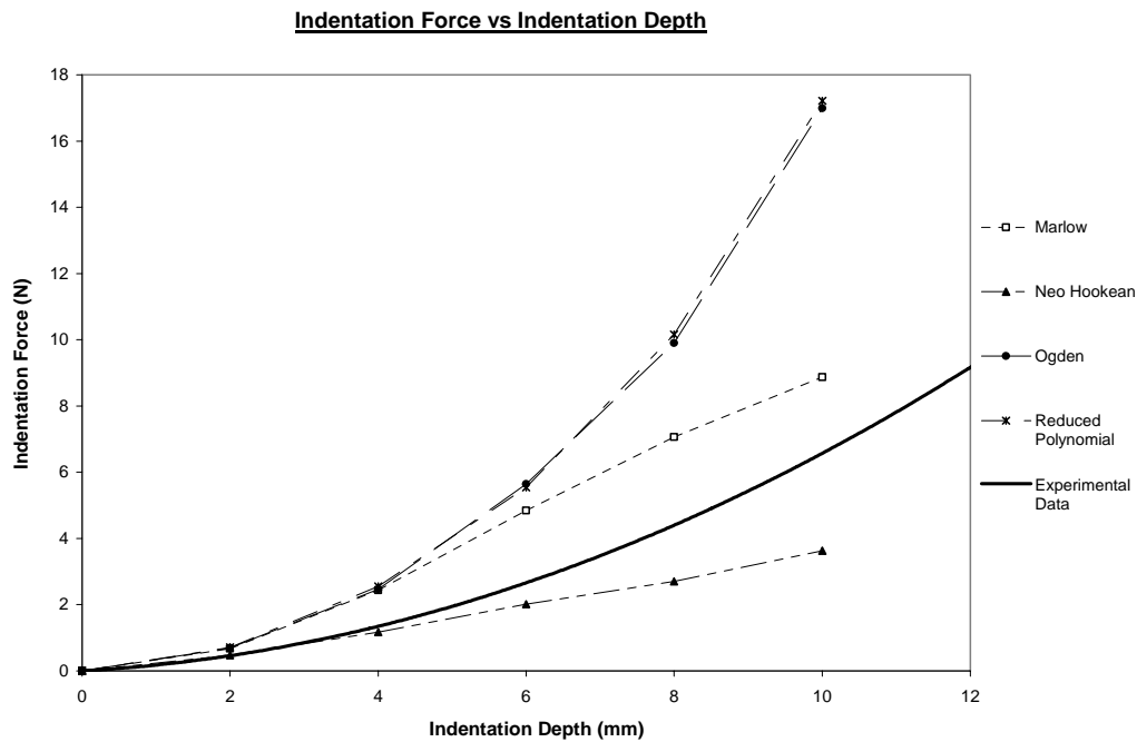
Figure 4.8. Graph of experimental and FE-predicted indentation reaction force against indentation depth for location 3,5 (distal popliteal region)
