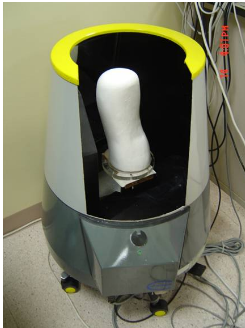
Figure 3.3. Positive mould of residual limb in CAPOD's prosthetic workstation
