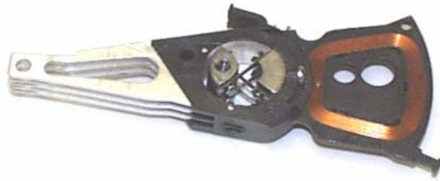
Figure 4.9: The assembly of a prototyped flexural pivot to an actuator arm.
