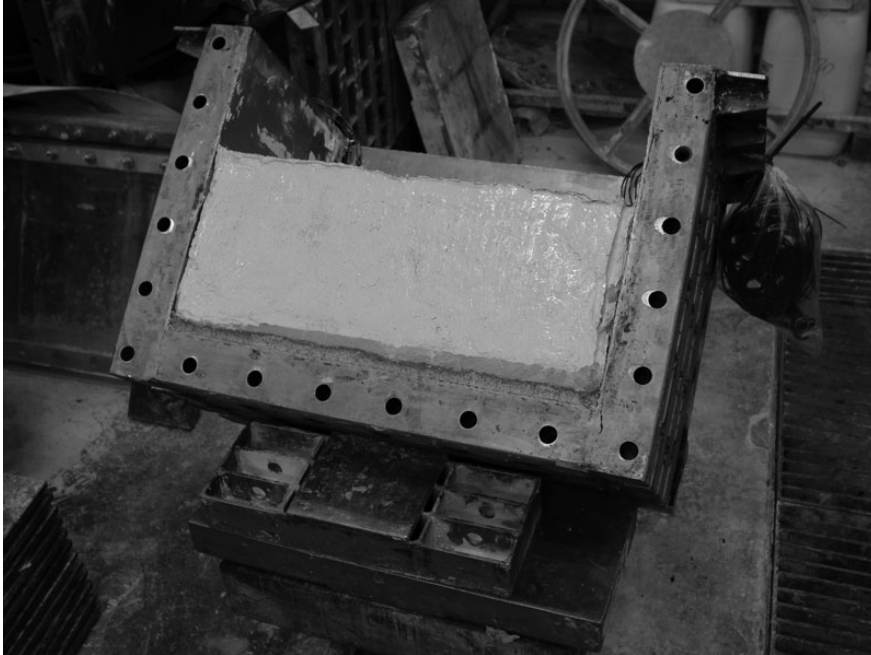
Fig. 3.31 Side wall of the model container were removed so that the model clay bed can be trimmed at prescribed levels using a wire cutter.
