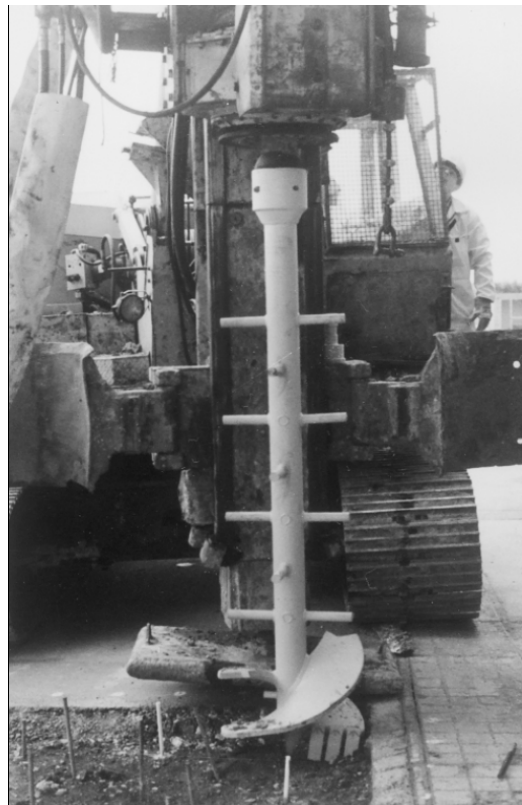
Fig. 1.8 The site trial prototype auger (Al-Tabbaa and Evans 1999).
