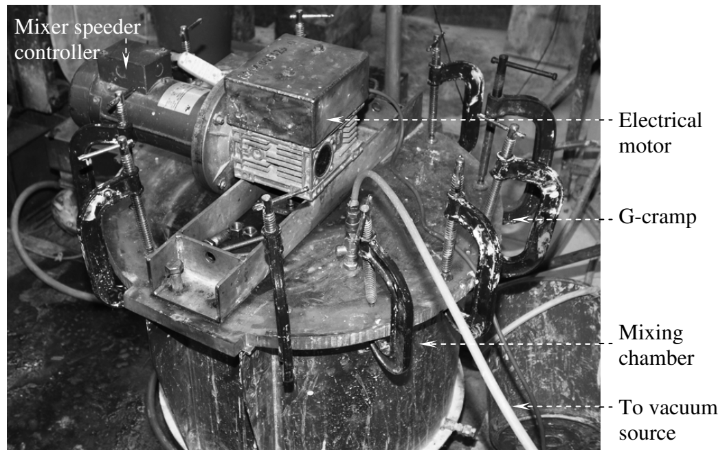
Fig. 3.27 De-aring chamber use in remoulding of the kaolin powder.
