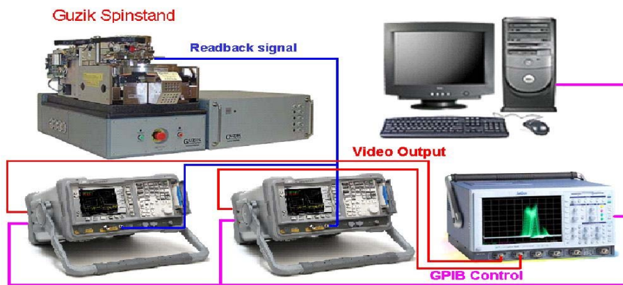
Fig. 4.8 Experimental setup for harmonic based in-situ fly-height and gap width measurement
