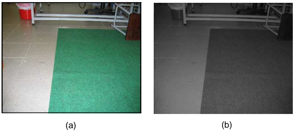
Figure 5.24: (a) Original 1280 x 1024 image (b) Resultant Image applied with Low pass filter
