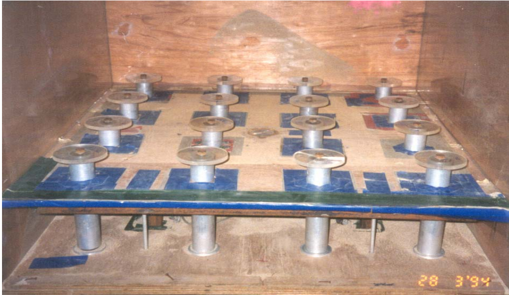
Figure 2.7 Experimental setup of piled embankments (after Tung, 1994)
