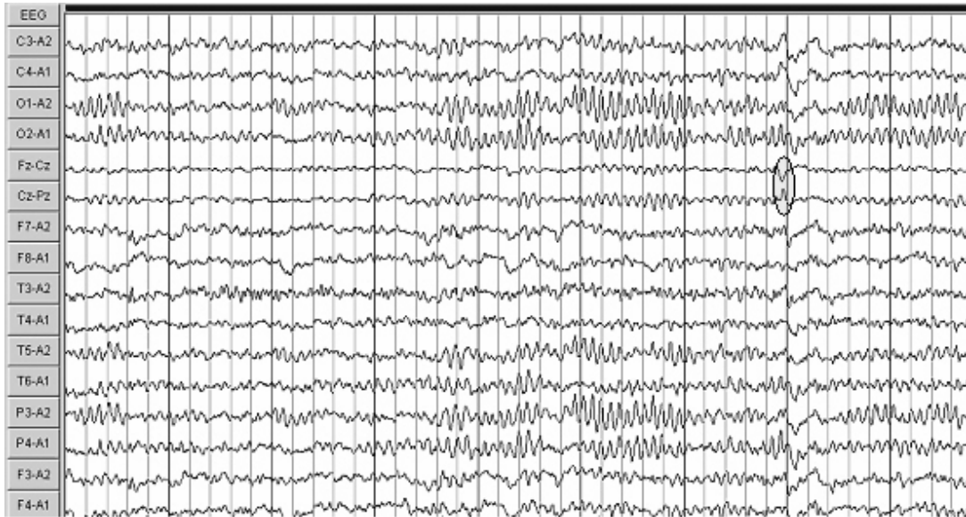
Figure 5.14 Raw EEG montage data (experiment pop2). Two vertexes were observed in Fz-Cz and Cz-Pz channels due to the pop sound stimulus at about 7th second.
