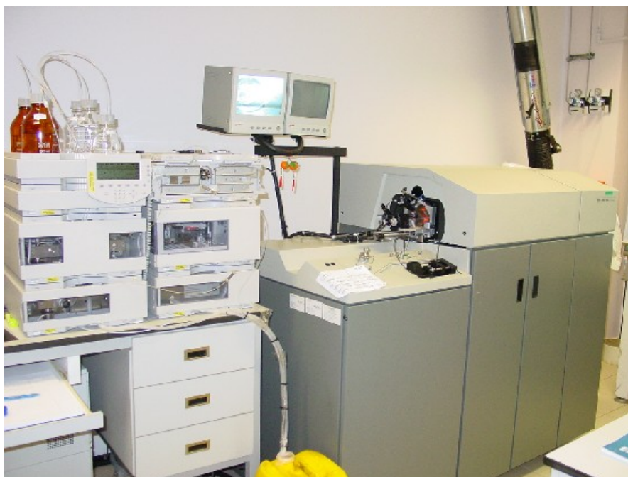
Figure 6: Agilent nano-flow LC-Qstar XL MS/MS system
