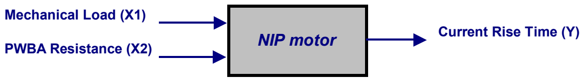
Figure 7.5: Schematic overview of relationship between PC and DP's.
