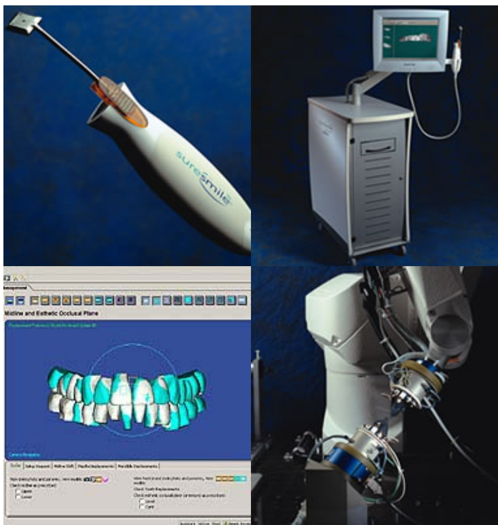
Figure 4.1 : the SureSmile® process: the scanner, the mobile scanner station, the simulation software, the arch-bending robotics
