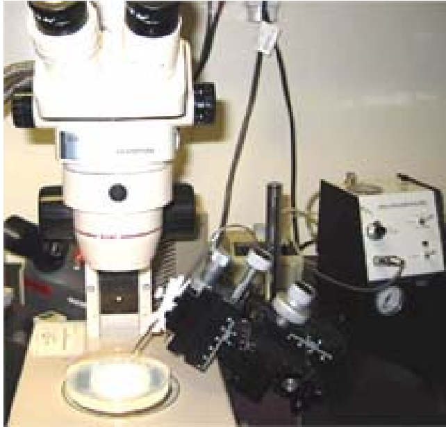
Fig. 2.2. Microinjection was performed using the MPPI-2 pressure injection system and dissection microscope Olympus SZ40.
