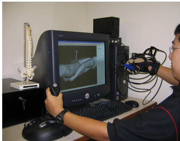
Figure 5.7 Overview of human-computer interaction in Virtual Spine Workstation
