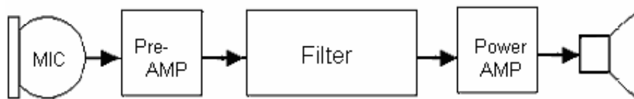
Fig. 1.2 An analog hearing aid system
