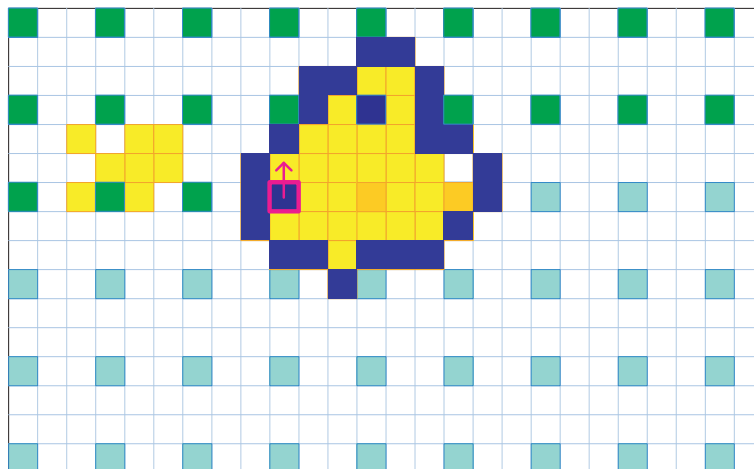
Figure 4.11: Back to step 1: next foreground pixel at coarse resolution level has been found
