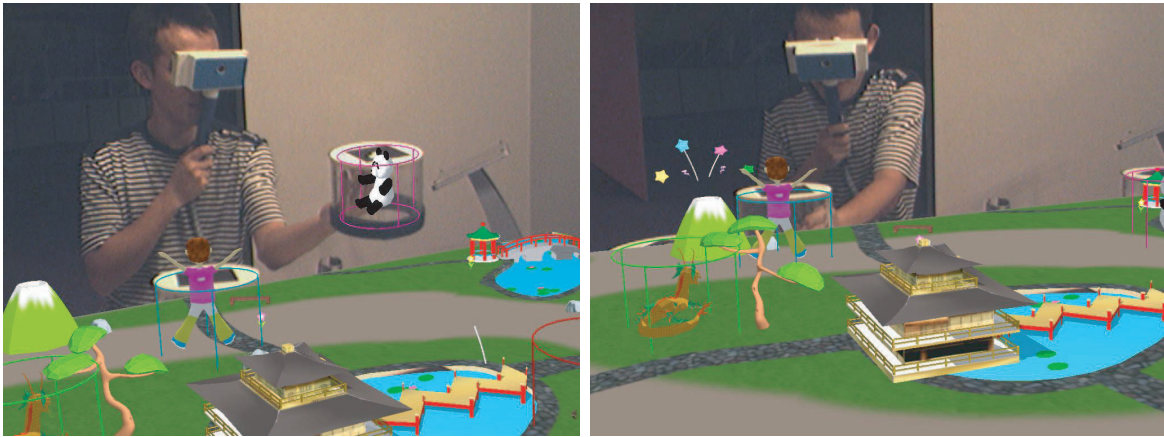
Figure 7.1: Tangible interaction on the Main Table: (Left) Tangibly picking up the virtual object from the table. (Right) The trigger of the volcano by placing a cup with virtual boy physically near to the volcano.
