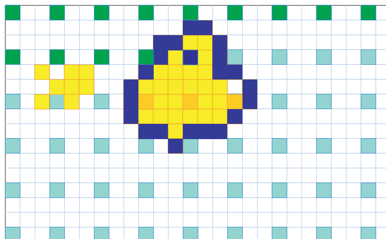
Figure 4.10: Step 4: Finish tracing all pixels of the contour
