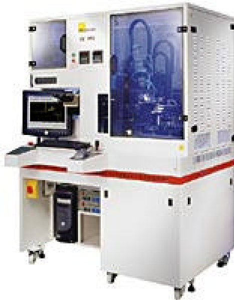
Figure 3.3 Photograph of Karl-Suss flip chip bonder
