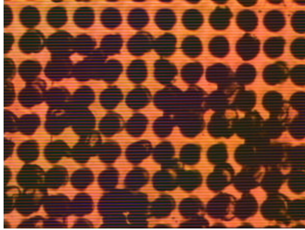
Figure 5.19 Optical micrograph of SU-8 residues in between the BoN interconnects after stripping
