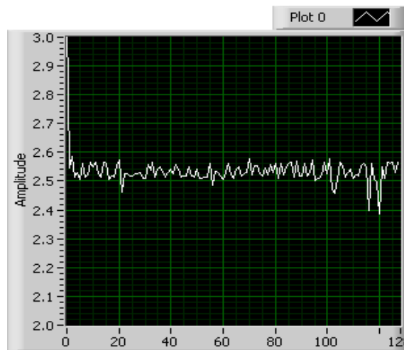
Fig. 6.20. The residual FPN readings of the first row of FPA.
