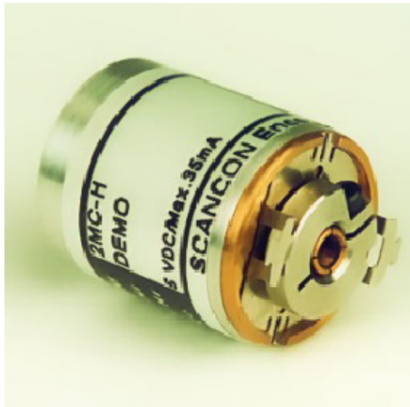
Figure F.1: Photograph of Scancon incremental encoder
