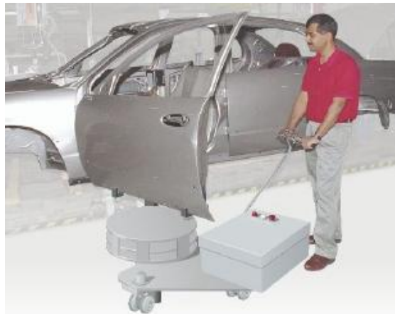
Figure 1.1. Industrial prototype of the Scooter cobot used at General Motors [6]
