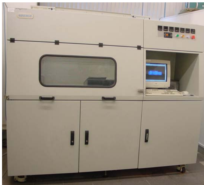
Figure 3.1 The NUS-developed experimental DMLS system
