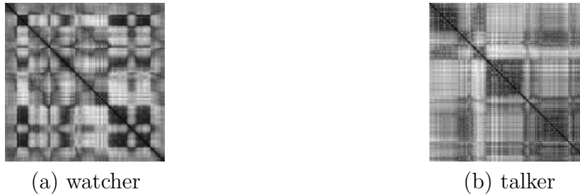
Figure 4.2: Similarity matrix R of a (a) watcher (exhibiting FCFA) and (b) talker (exhibiting focused attention).
