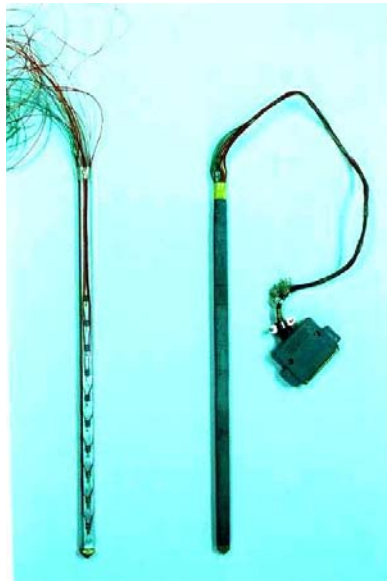
Figure 3.4 A partially completed and a completed model pile
