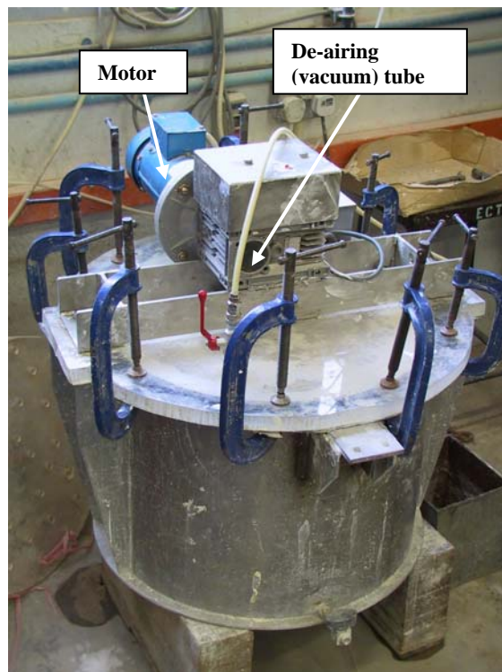
Figure 3.14 De-airing mixer used to mix and de-air kaolin clay
