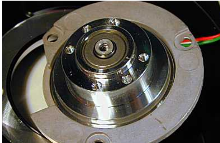
Figure 5.2: A hard disk spindle motor
