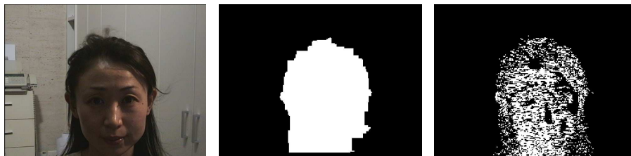
Figure 5.30: A Japanese human subject, binarized ROI and the skin color probability diagram
