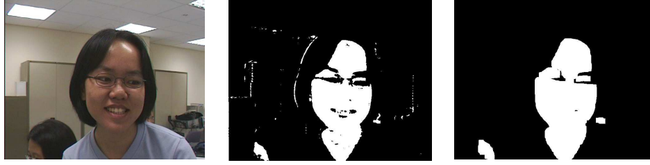
Figure 5.21: (a)source image (b)after median filtering (c) after morphological operations
