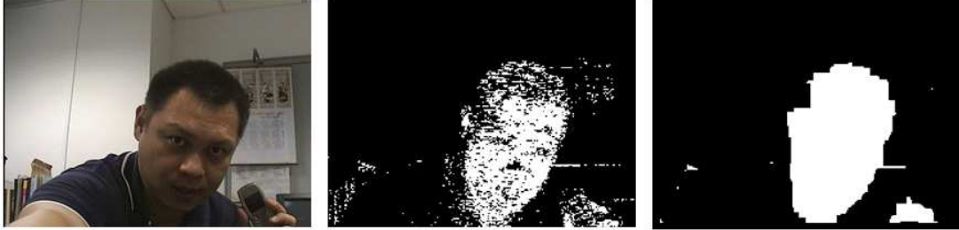
Figure 3.9: Filtering by Morphological Opening Operations
