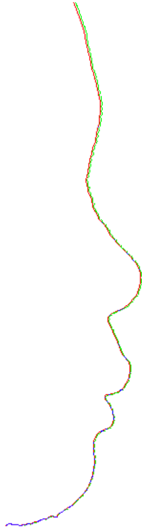
Figure5.8: The registration result of the two facial profiles. (green: image I' ; red: image I ; blue: the common part of the two images)
