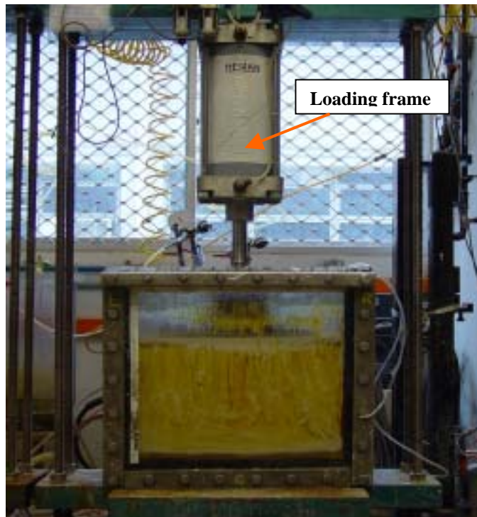
Figure 3.7 Sample preconsolidation in the loading frame
