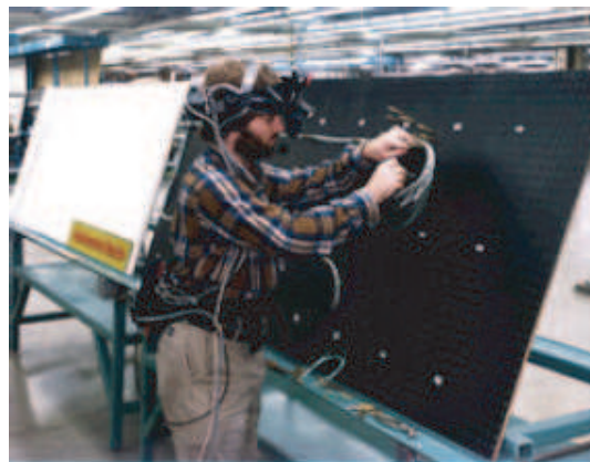
Figure 2.5: Adam Janin demonstrates Boeing's prototype wire bundle assembly application.
