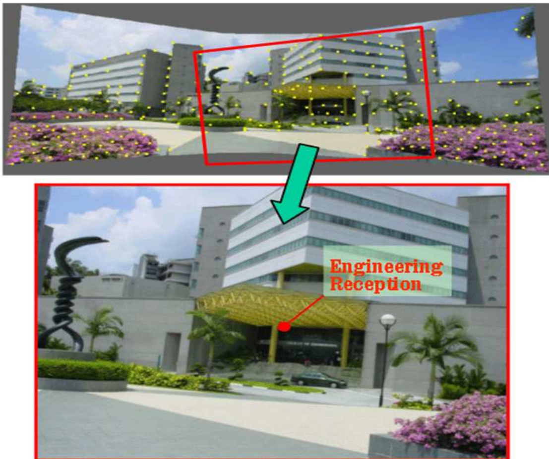
Figure 5.2: Information for geographical annotation can be stored in the form of corner points and surrounding regions and their directions in space. These points may be stored at a given point across a wide range of angles (displayed top as a mosaic). The input frame (bottom) can be compared to this stored representation to establish the position of the label.
