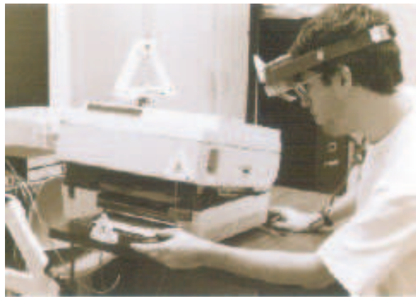
Figure 2.3: External view of Columbia printer maintenance application. Note that all objects must be tracked.
