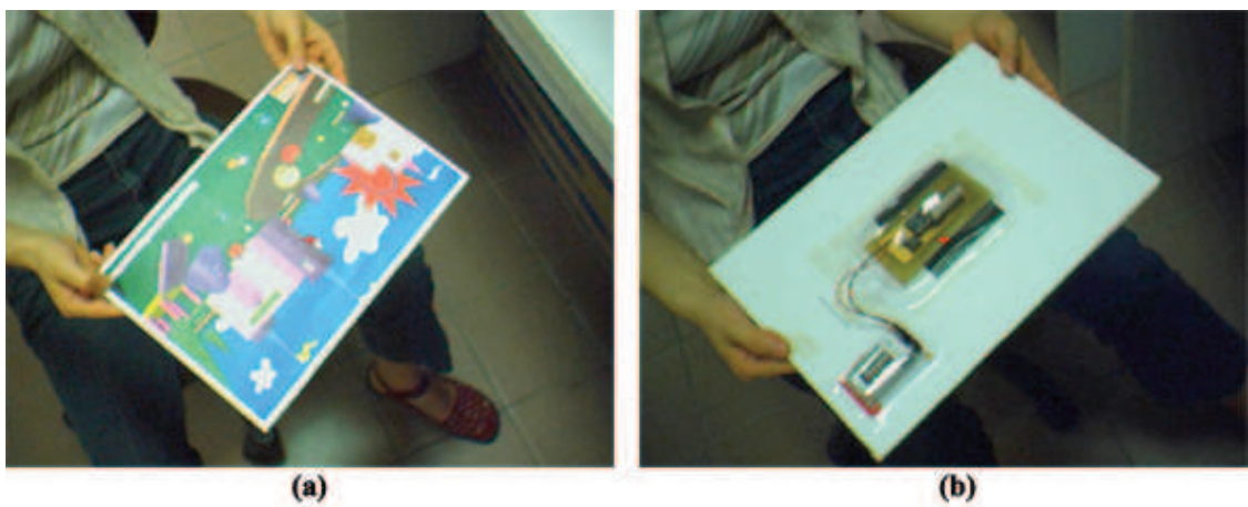
Figure 5.9: The board used in the Pacman game application. (a) The front view of the board: the colorful page to be tracked is pasted here. (b) The rear view of the board: the tilt pad is mounted here.
