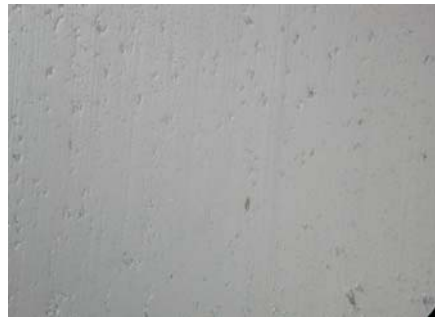
(c) Ductile mode (#4000, R_a: 0.009 \mu m )
