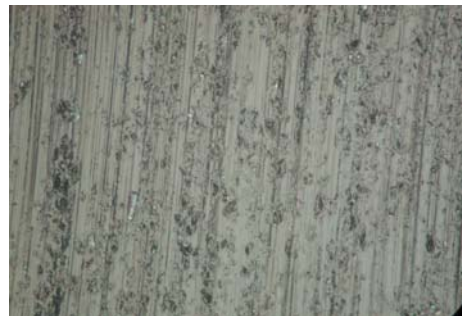
(d) Without ELID (#1200, R_a: 0.184 \mu m ) (e) With ELID (#1200, R_a: 0.099 \mu m )
