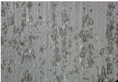
(d) Without ELID (#1200, R_a: 0.184 \mu m ) (e) With ELID (#1200, R_a: 0.099 \mu m )
