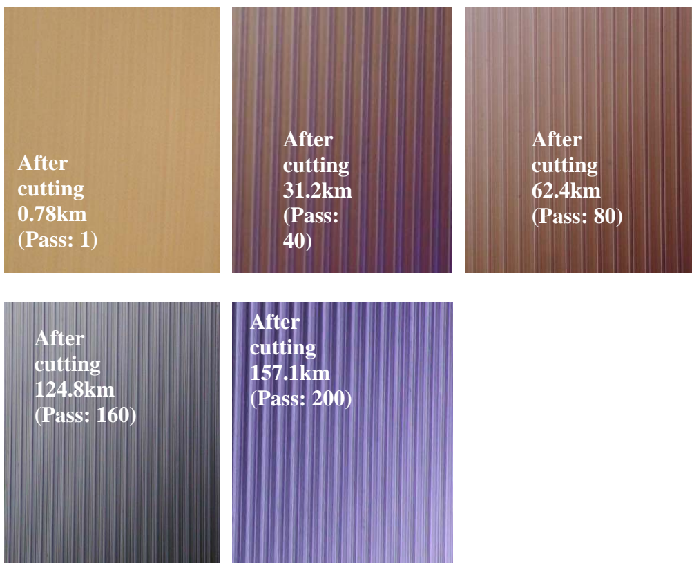
Figure 5.27: Surface for cutting EN of %P (w/w)=11.5, at different cutting distance
