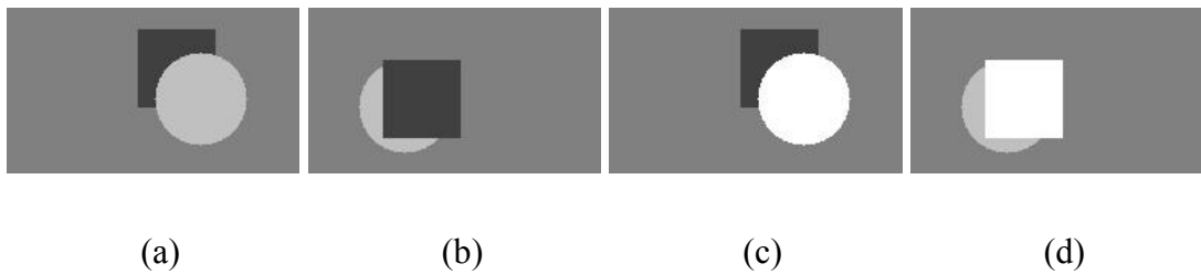
Figure 5.2 Illustration of hypothesized measurements. (a) (b) Two frames of the “rectangle and circle” sequence under different occlusion relationships. (c) Masked image under the first occlusion hypothesis. (d) Masked image under the second occlusion hypothesis.
