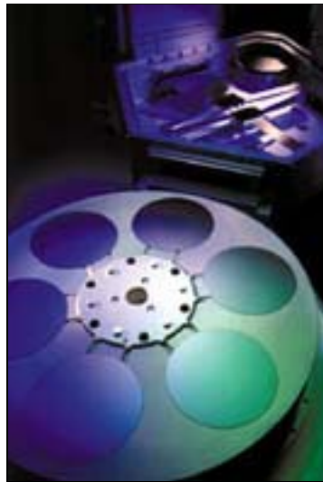
Picture 3- 1 Multi-station of Concept two Sequel Express PECD system (courtesy of Novellus System Inc.)
