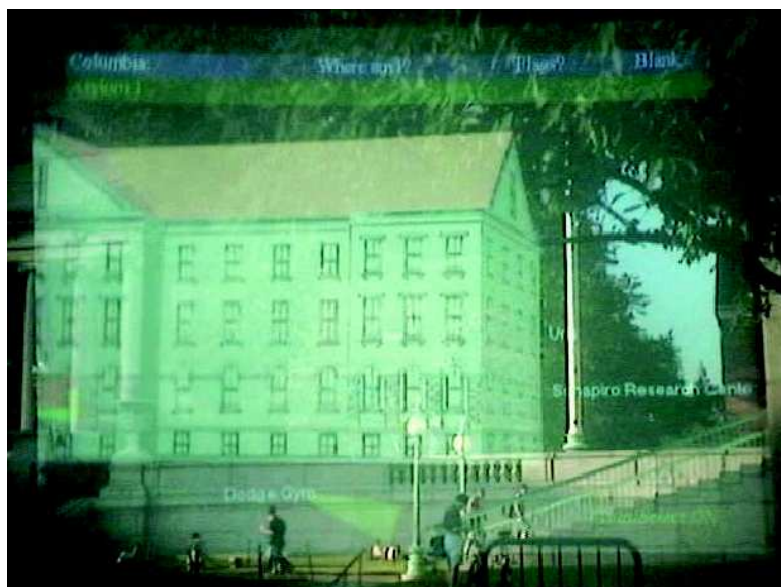
Figure 2.8: A View Through a SeeThrough HMD Shows a 3D Model of Demolished Building at Its Original Location. (Image used with permission, courtesy of Prof. Steven Feiner, Computer Graphics and User Interface Lab, Columbia University.)
