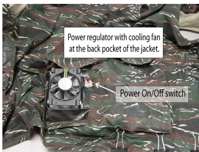
Figure 3.12: Power Regulator at the Back Pocket.
