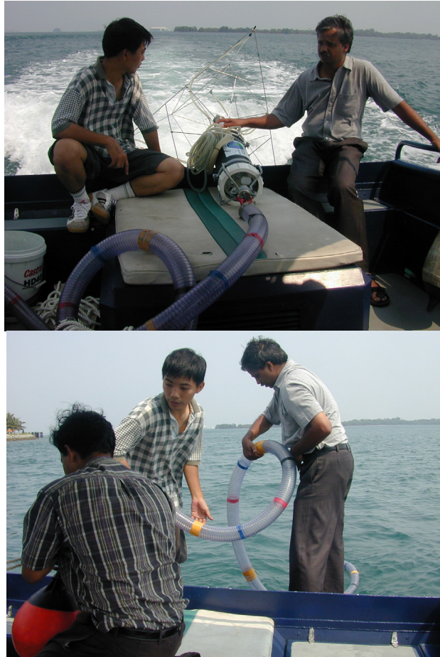
Figure 39: Deployment of HiDAQ using a tubular spar-buoy
