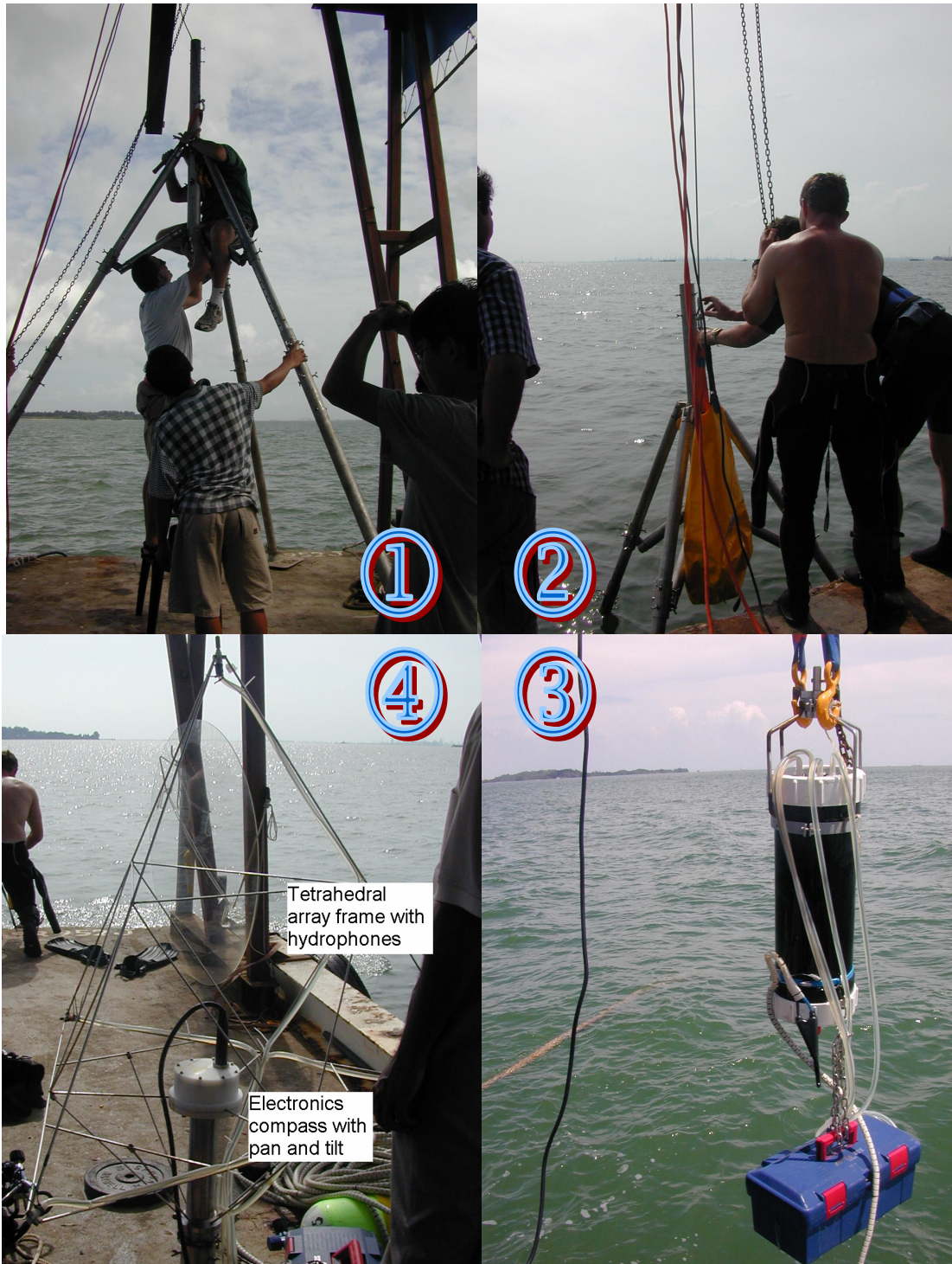
Figure 40: Deployment of HiDAQ in bottom-mounted configuration from a barge
